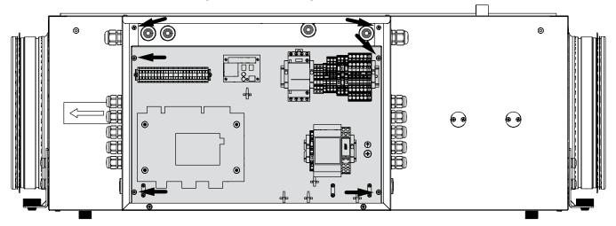
Connect all cables inside the unit in the new location at the same points as before disassembly. Reinstall the control unit cover.
