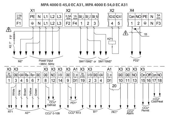
The interpretation of the designations and the characteristics of the connection cables are given in the table.
