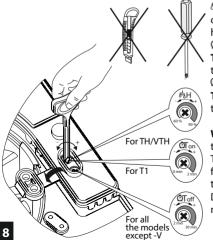
&H To adjust the humidity set point turn the control knob **H** clockwise to increase and counter-clockwise to decrease the humidity sensor set point, adjustable from 60 % up to 90 %.
